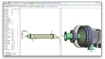
Kettle floating head heat exchanger with eccentric cone.
